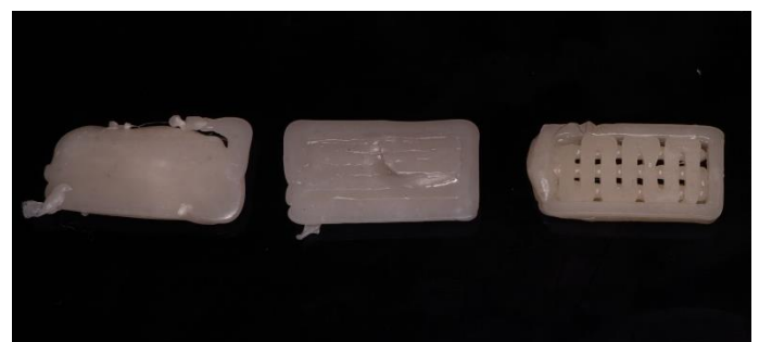
Fig 1: Scaffolds made using pneumatic extrusion
